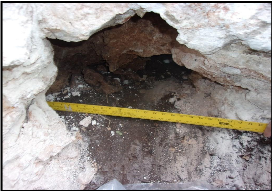
Photo 8. Feature S-8 horizontal dimension (21 inches) of the horizontal solution cavity in the excavation sidewall.
