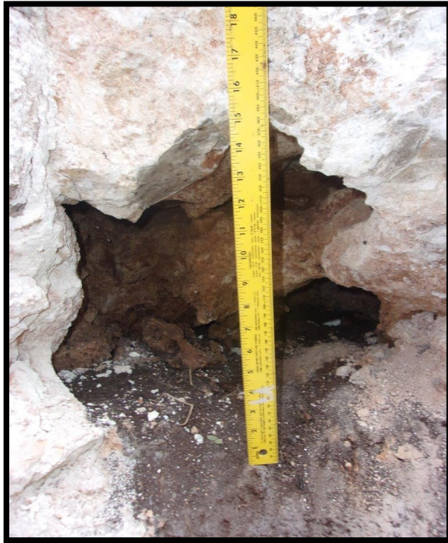
Photo 7. Feature S-8 vertical dimensions (14 inches) of the horizontal solution cavity in the excavation sidewall.
